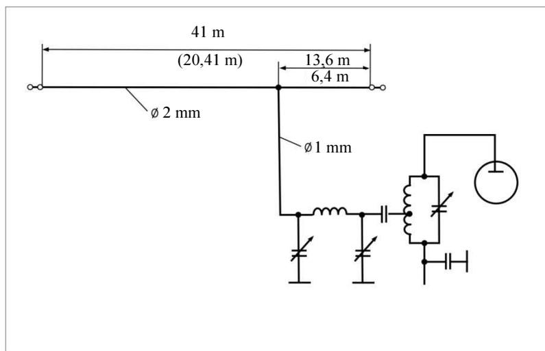
The next modification of Windom antenna was antenna made by German radio amateur with call sign DL1BU (*Günter Schwarzbeck, editor's note*) in 1950, who fed it with a balanced feeder.
