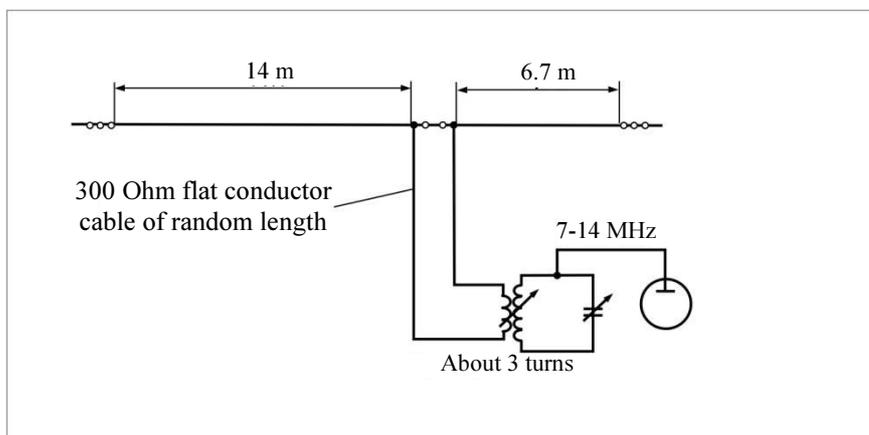
The German did find a gap in the above zero-reactance point, and connected the balanced line with characteristic impedance of 300 Ohms. That feeding system ensured greater symmetry and stability of the impedance, as opposed to a single-wire feed-line, which, in addition, produced significant radiation. A two-wire feed-line radiates significantly less, which contributes to the stability of the radiation pattern and settings.
