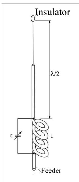
However, this circuit is narrowband, and provides operation on a single band only. Being in possession of modern fleet of measuring instruments and sufficient number of ferrite cores, I set out as a goal to manufacture a broadband current choke with a level of isolation up to 30 dB, and operating band of 3-30 MHz. And that choke was successfully made.
