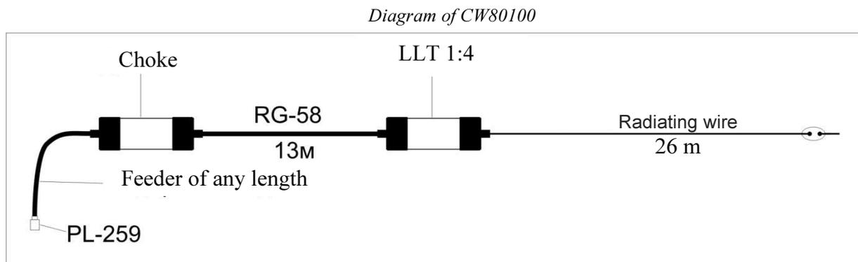
Thus, unlike all previous versions of the Windom antenna, a new antenna called City Windom has a new advantage, it's a feed-line at the same time as being a radiator. This makes it possible to get along with only two attachment points instead of three, which significantly improves user performance and usability of the antenna in modern urban environment.
