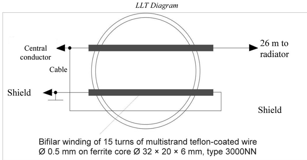
Here the energy is transferred over a two-wire feed-line. The magnetic field transfers solely the asymmetrical currents.
