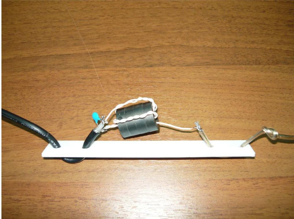
in which the short section (13.5 m) was made from a coaxial cable. Following it, the abovementioned choke was installed. All measurements were performed on the choke output connector. Predictably, we managed to separate the radiator from the feeder, and I began to observe on the instrument the clear resonances of all 6 bands 80-40-20-17-12 and 10 meters.
