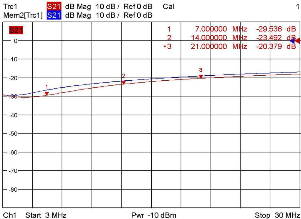
Here are two graphics. The blue line shows the isolation on the ferrite of brand 3000NN, and the red one shows the same on 1500NN brand.
